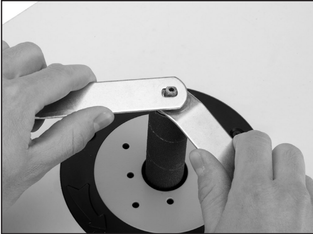
Figure 8. Loosening the spindle hex nut.
